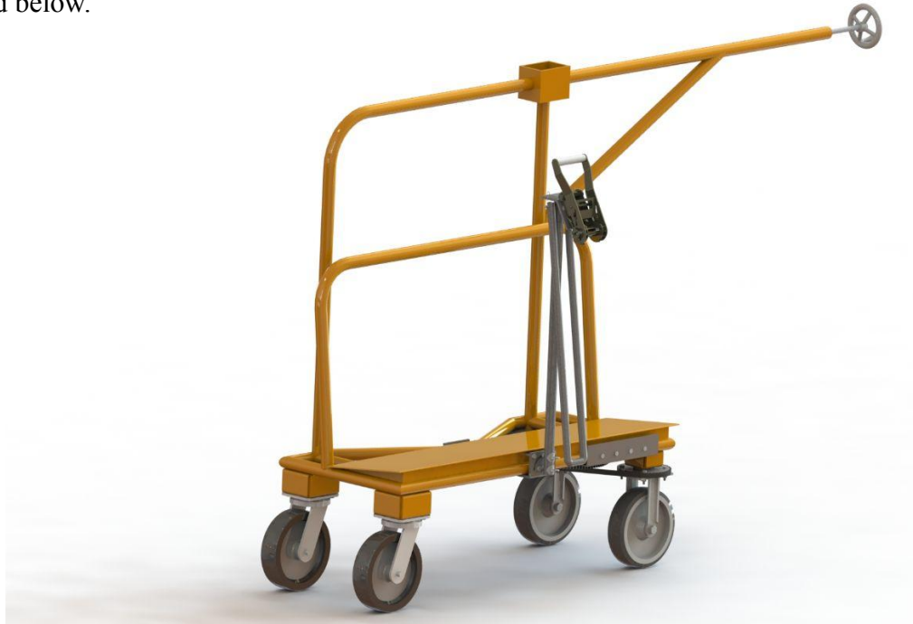
Figure 4: Final CAD model of our drywall cart design
