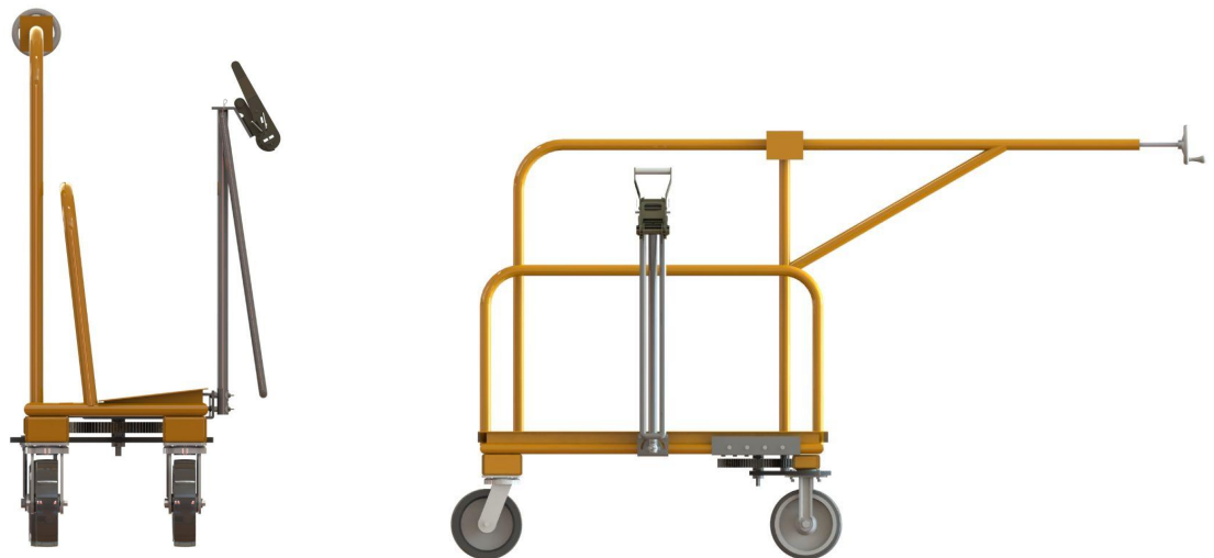
Figure 4a: Final CAD model of our drywall cart design
