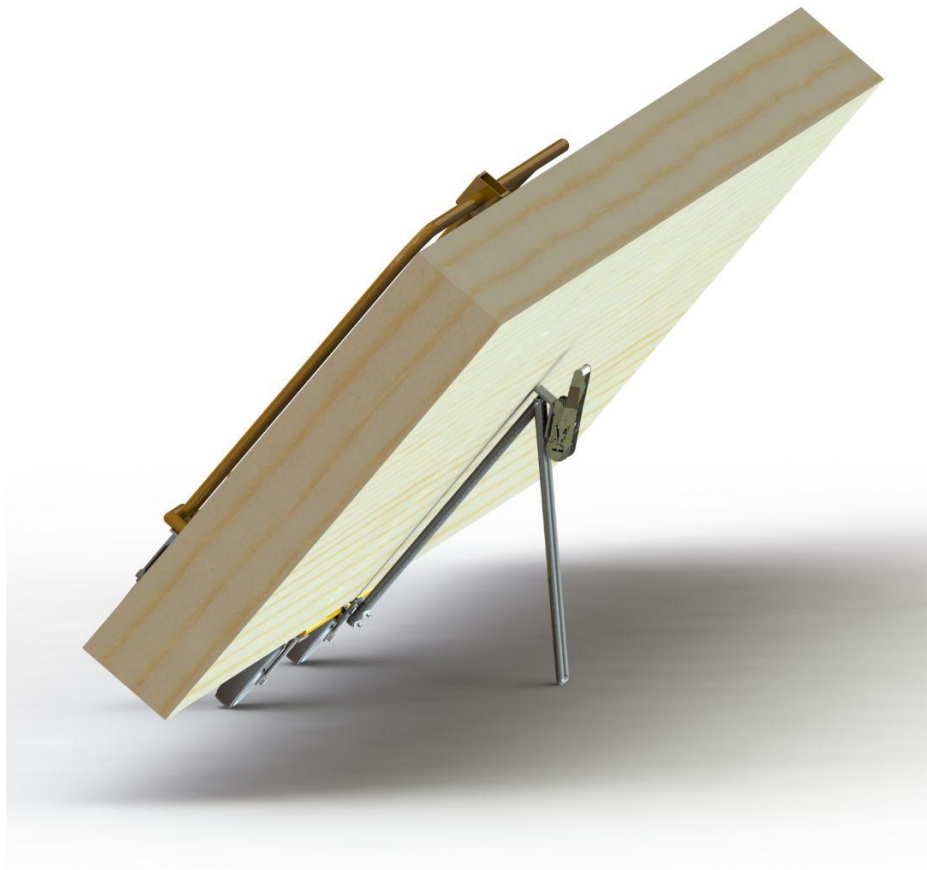
Figure 10: Model Rendering of deployed kickstand
